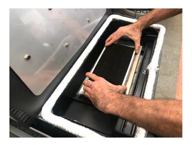
6. Install the new combustor. Make sure the weld around the perimeter of the stainless steel flange is facing UP. The flange is welded around the combustor at an angle. The combustor should be installed so the face is directed forward with the short edge at the front, and the tall edge at the back. This position directs the heat produced by the catalyst forward.
